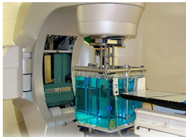
SMARTSCAN automates and guides the physicist through the beam scanning and commissioning. Image Courtesy of University Hospitals Bristol NHS Foundation Trust, UK.
